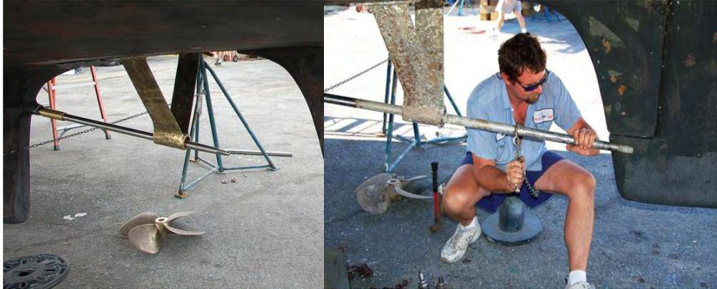
This spring checkup revealed the need for a new shaft, cutlass bearings, and reconditioning of the prop. This is more than routine yearly maintenance. Camachee Cove Yacht Yard worker removing shaft during spring maintenance.
