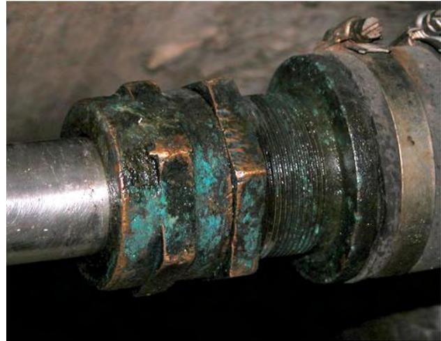
Check shaft inside boat, shaft log and stuffing box. Replace stuffing if needed.
