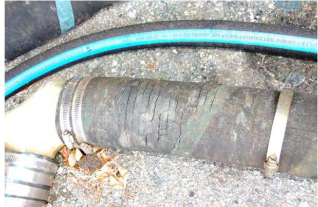
Check hoses for cracking or other signs of deterioration.
